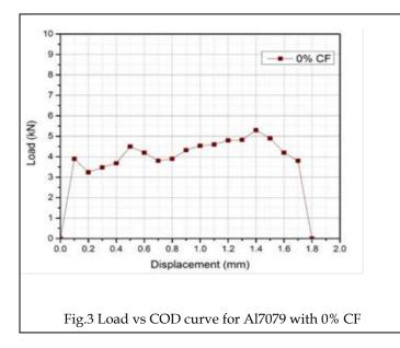
From the Fig. 3, the values of critical load 'Pq' and 'Pmax' is found to be Pq= 4.82kN and Pmax = 5.3kN. For the nondimensional term, a/W=12.994/25.4=0.511, the corresponding geometrical correction factor recommended by ASTM E399 standard table (Appendix A) was found to be 9.96. By using the equations 1 to 5 for plain strain fracture toughness, the value of Kq is tabulated in the table 1.
