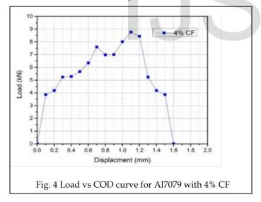
From the Fig. 4, the values of critical load Pq= 8.0kN and Pmax = 8.76kN. For the non-dimensional term, a/W=12.994/25.4=0.511, the corresponding geometrical correction factor recommended by ASTM E399 standard table (Appendix A) was found to be 9.96. The value of Kq is tabulated in table 1.
