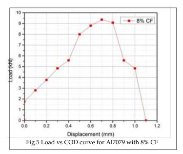
From the Fig. 5, the value of critical load and maximum load is Pq = 8.8kN and Pmax = 9.36kN. For the non-dimensional term, a/W=12.994/25.4=0.511, the corresponding geometrical correction factor recommended by ASTM E399 standard table (Appendix A) was found to be 9.96. The value of Kq is tabulated in table1.
