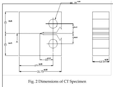
The general expression of the plain strain fracture toughness for a CT specimen made up of Aluminum 7079,
